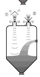
> The instrument cannot be installed in the arched or domed roof intermediate. In addition to produce indirect echo is also affected by the echoes. Multiple echo can be larger than the real value of signal echo, because through the top can concentrate multiple echo. So cannot be installed in a central location.
