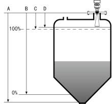
**Datum measurement:** Screw thread bottom or the sealing surface of the flange.
